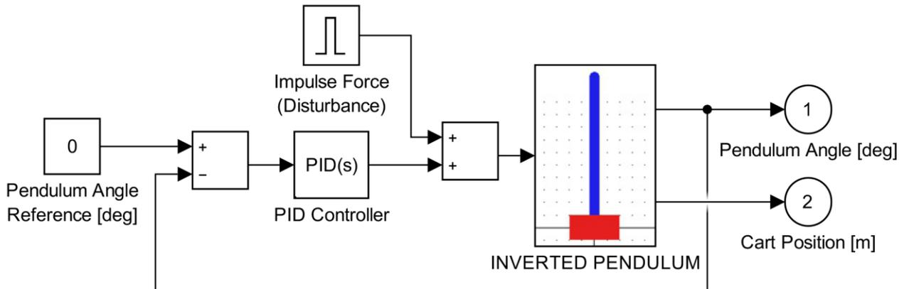
**Figure 4. PID control block diagram of Inverted Pendulum**
