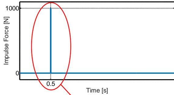
**Figure 5. 1-Nsec impulse disturbance applied to the cart**
