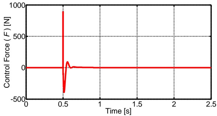
Figure 9. Control Force of PID controlled system
