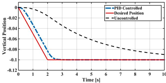
Figure 6. Vertical position control of Scara type 3D printer.
