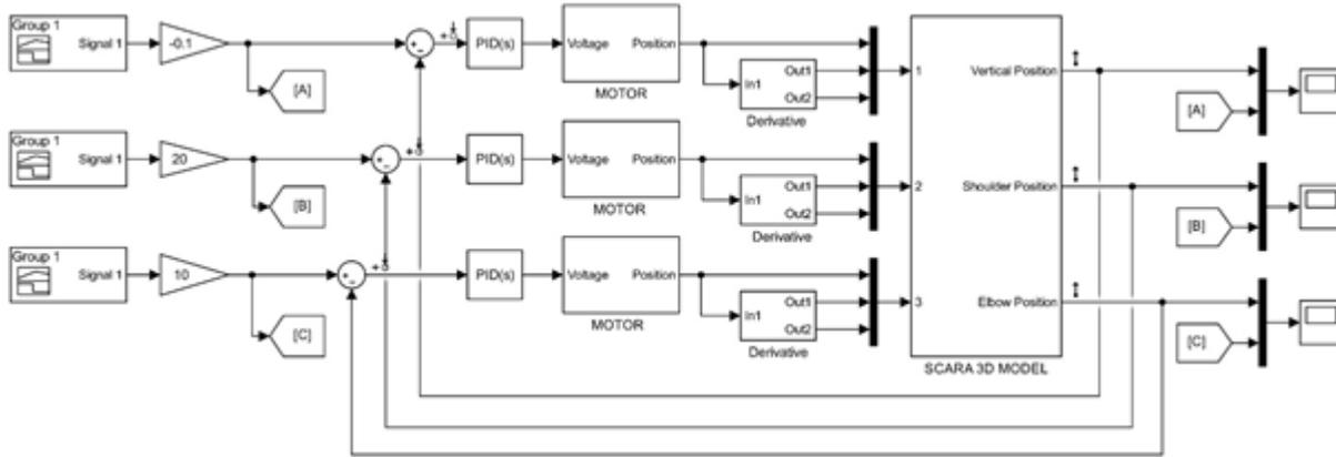
Figure 2. MATLAB/Simmechanics model of Scara type 3D printer.
