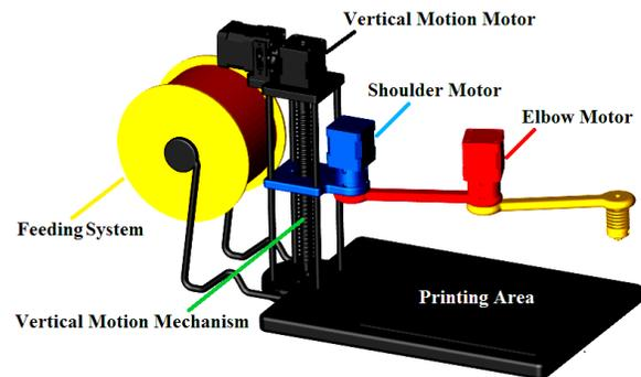
**Figure 1.** MATLAB/Simmechanics model of Scara type 3D printer.
