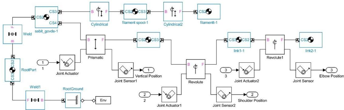
Figure 5. MATLAB/Simmechanics model of Scara type 3D printer.
