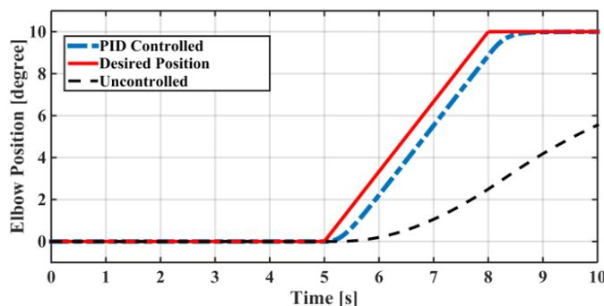
Figure 8. Elbow position control of Scara type 3D printer.
