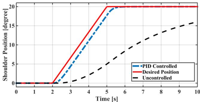
Figure 7. Shoulder position control of Scara type 3D printer.
