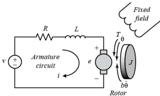
Figure 4. Free body diagram of the DC Motor
