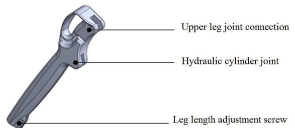
Fig. 4. Lower leg Cad model.
