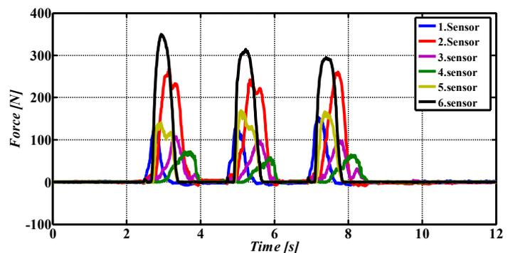
Fig. 9. Measured data from shoe sensors along a walking cycle.
