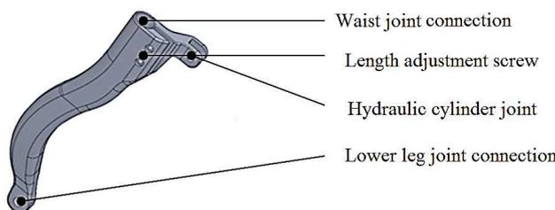
Fig. 3. Upper leg Cad model.
