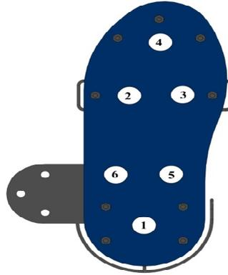
Fig. 6. Force sensor layout.
