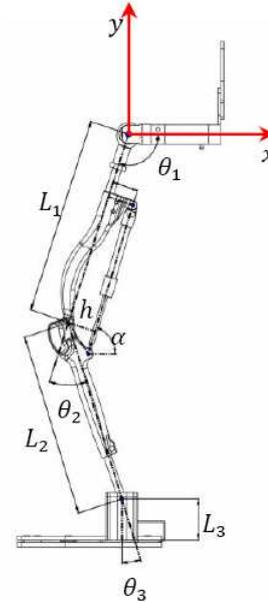
Fig. 1. 3D-Cad model of designed exoskeleton system. Fig. 2. The schematic picture of exoskeleton mechanism.
