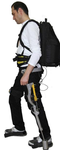
Fig. 2. Lower extremity exoskeleton system
